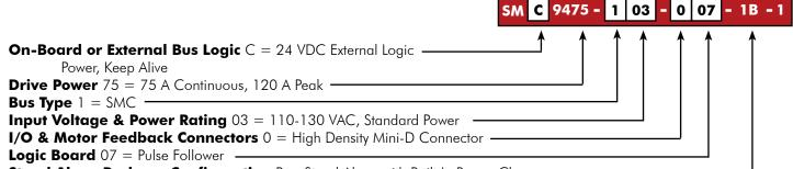
Stand Alone Package Configuration B = Stand Alone with Built In Regen Clamp
