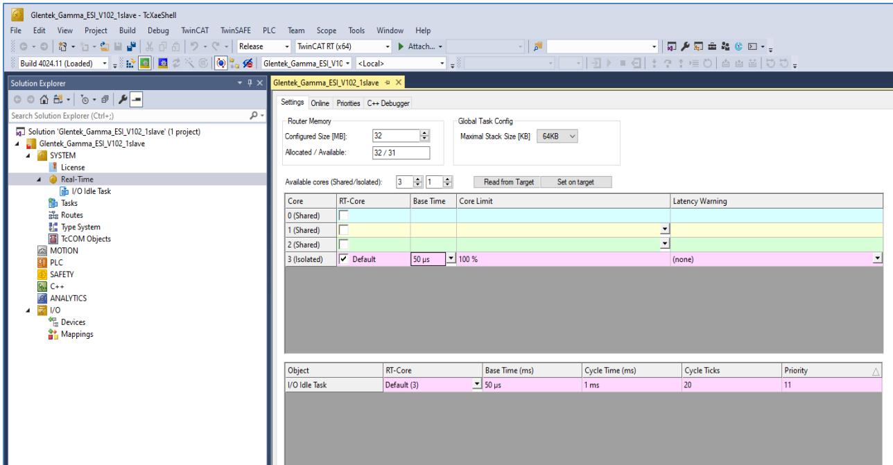
**Figure 15 - 2. Set-up Real-Time with the Isolated Core**
