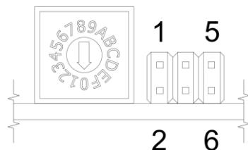
**Figure 4 - 3. EtherCAT ID Selector (Rotary SW and Jumper)**
