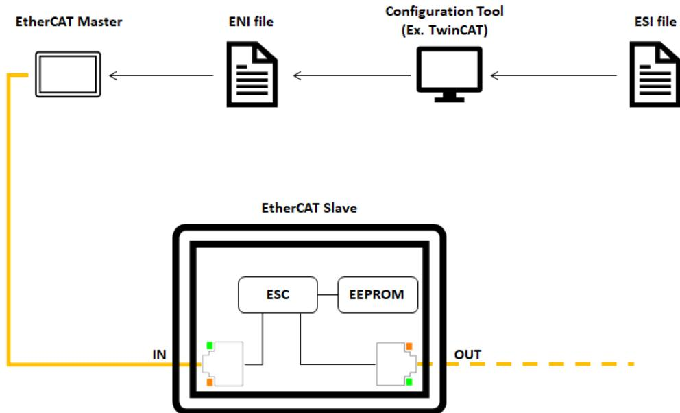
Figure 3 - 3. EtherCAT System Architecture
