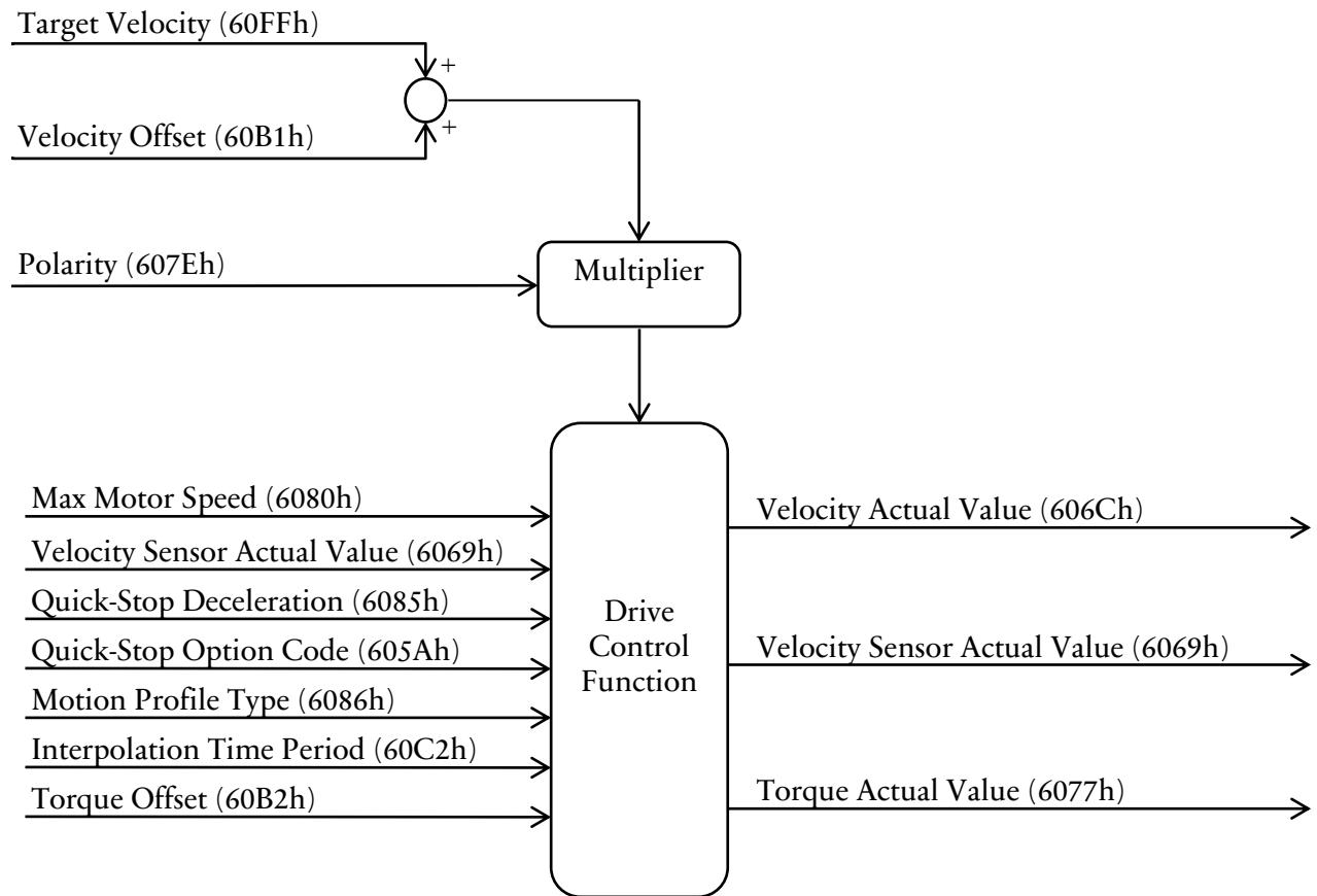
**Figure 10 - 2. Cyclic Synchronous Velocity Control Function**
