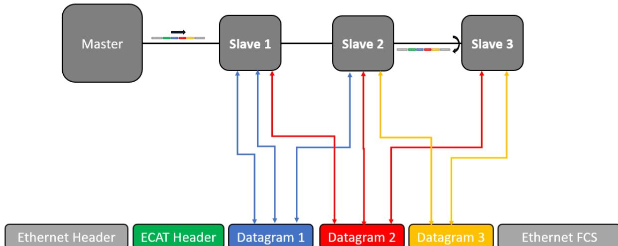
Figure 3 - 2. Inserting data on the fly
