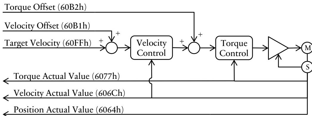
Figure 10 - 1. Cyclic Synchronous Velocity Mode Overview
