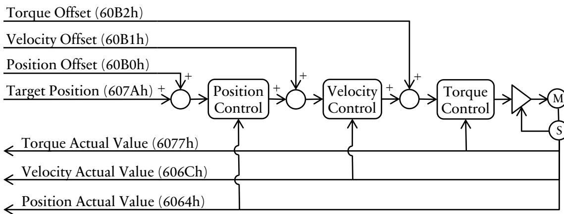
Figure 9 - 1. Cyclic Synchronous Position Mode Overview
