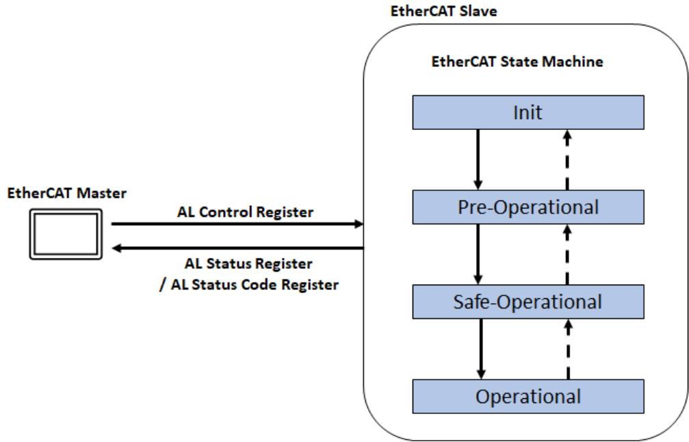
**Figure 3 - 4. EtherCAT Slave State Machine**
