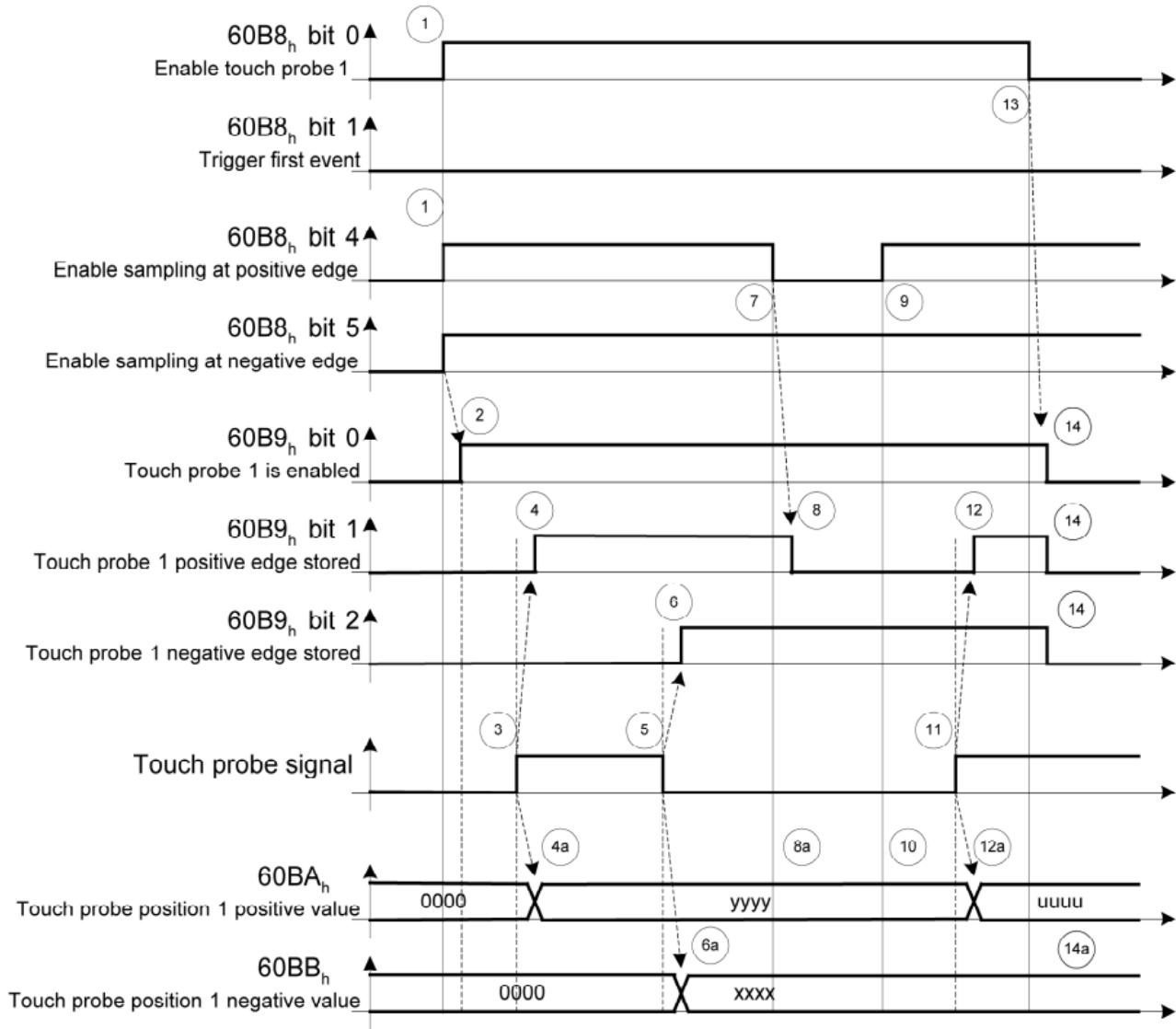
Figure 8 - 2. Timing Diagram for Touch Probe Example
