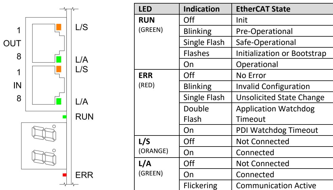
Figure 4 - 1. The EtherCAT port of the Gamma Drive (RJ45)
