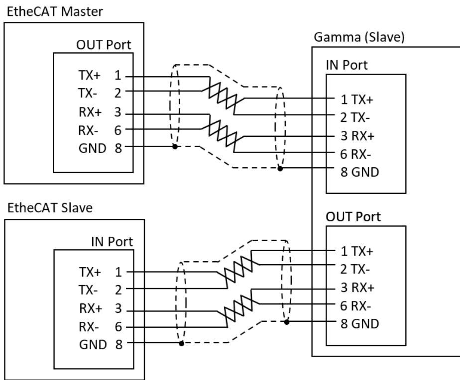
**Figure 4 - 2. The EtherCAT Connection Diagram**
