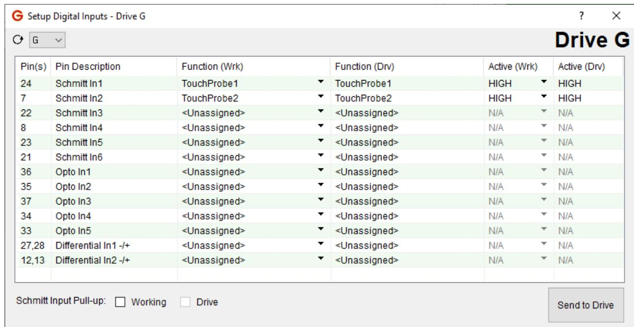
Figure 8 - 1. Example of Assigning Touch Probe 1 and 2
