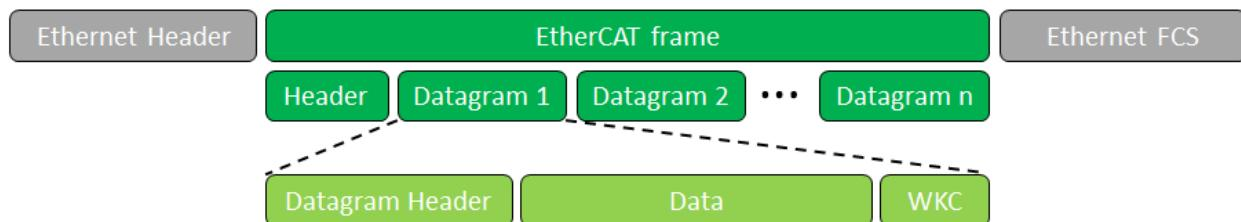
Figure 3 - 1. EtherCAT in a standard Ethernet frame (according to IEEE 802.3)
