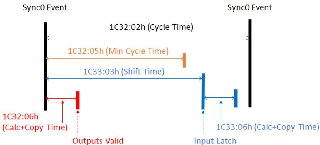
**Figure 14 - 2. Sync0 Synchronization Mode**
