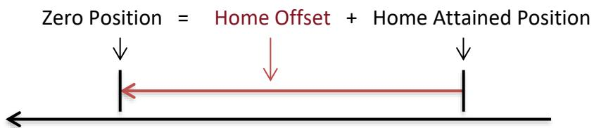
Figure 7 - 35. Setting Zero Position Utilizing Home Offset
