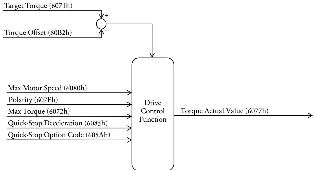
**Figure 11 - 2. Cyclic Synchronous Torque Control Function**
