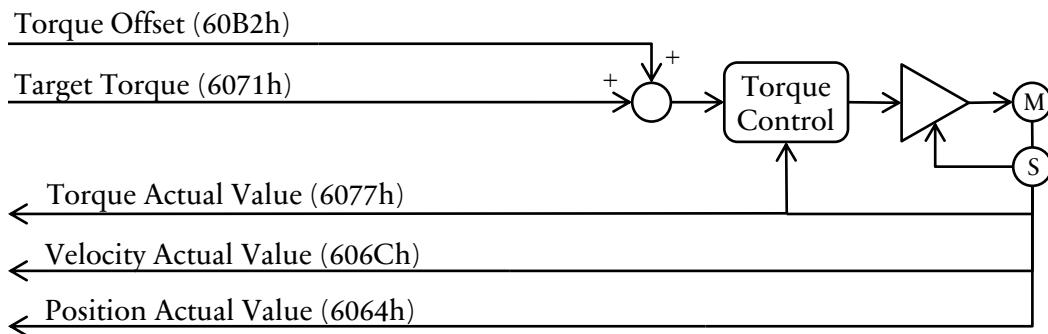
Figure 11 - 1. Cyclic Synchronous Torque Mode Overview
