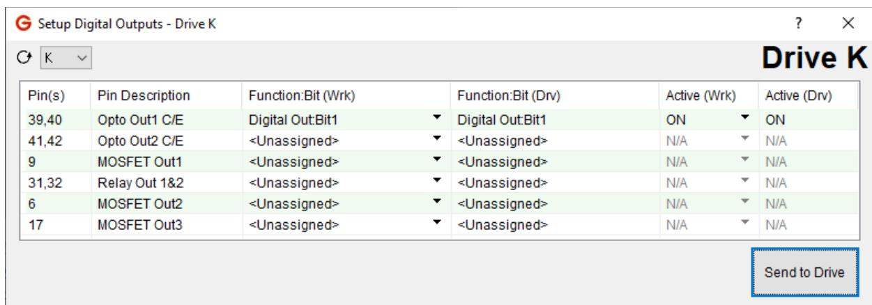
**Figure 16 - 1. Example of Assigning Digital Outputs**
