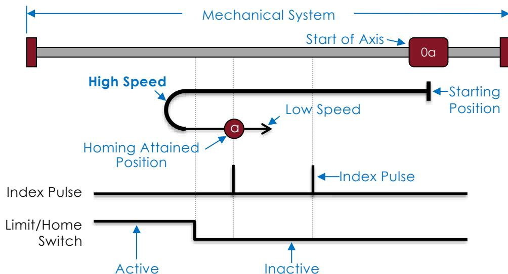
**Figure 7 - 2. Key Components for the Homing Diagrams**
