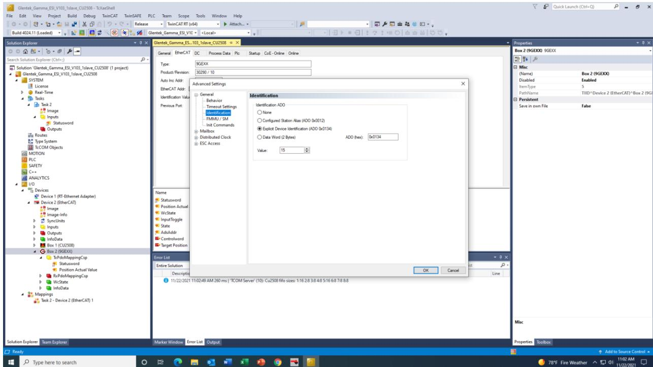
Figure 4 - 4. Set Explicit Device Identification by TwinCAT
