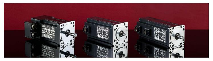
Glentek's GMB3500 series of high performance, permanent magnet Brushless servo motors utilize high-energy Neodymium-Iron- Boron (NdFeB) magnets, which provide more torque in a smaller package with higher dynamic performance than traditional ferrite magnet designs. In addition, due to high torque to inertia ratio of these motors, they are ideal for applications which require high acceleration and deceleration characteristics or where the physical size of the motor is a major concern.
