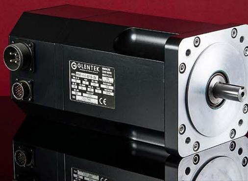
Glentek's GMB5600 series of high performance, permanent magnet Brushless servo motors utilize high-energy Neodymium-Iron- Boron (NdFeB) magnets, which provide more torque in a smaller package with higher dynamic performance than traditional ferrite magnet designs. In addition, due to high torque to inertia ratio of these motors, they are ideal for applications which require high acceleration and deceleration characteristics or where the physical size of the motor is a major concern.
