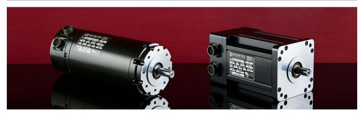
Glentek's GMBF4300 series of high performance, permanent magnet Brushless servo motors utilize traditional ferrite magnets which are ideal for cost sensitive applications. This helps to reduce the mechanical shaft resonance which allows higher servo gains with increased stability. In addition, all frame sizes incorporate skewed stators which provide ultra smooth operation (i.e. low cogging torque) at all speeds.
