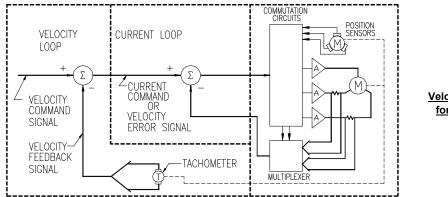
Figure 2.2b <u>Velocity mode sevo loop</u> <u>for a brushless motor</u>
