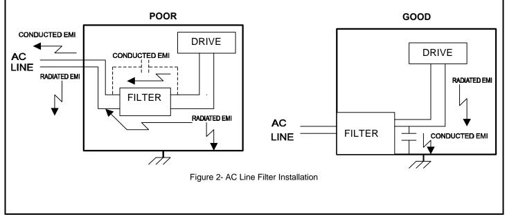
When multiple power cables enter an enclosure, an unfiltered line can contaminate a filtered line external to the enclosure. Therefore, all lines must be filtered to be effective. The situation is similar to a leaky boat. All the holes must be plugged to prevent sinking.
