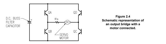
The advantage of an "H TYPE" output bridge configuration is that by controlling the switching of the opposite pairs of transistors, current can be made to flow through the motor in either direction using a single-polarity power supply.
