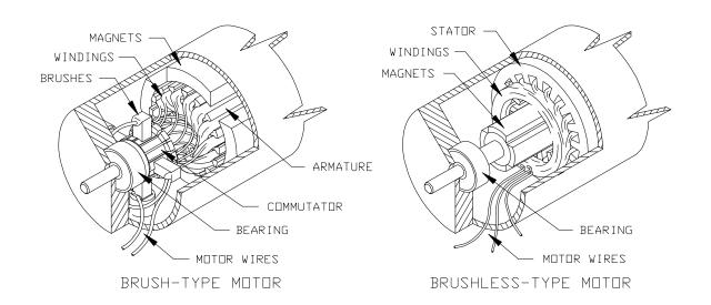
Figure 2.3 Brush type and Brushless type Motors
