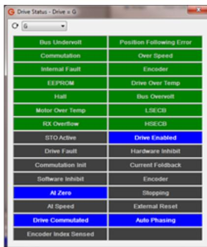
9. Verify that the motor phase wires are connected properly, number of poles (this is not pole pairs), and line per revolution (not the quadrature count) are set correctly. If all were correct, increase *Final Current* value to 60% of motor rated current. Click on Send Settings to Drive. Click on Tools -> Control Panel. Click on Fault Reset in the Control Panel dialog to clear all faults.
